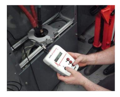
HVPD pC (picocoulomb) Calibrator is a handheld unit suitable for calibration pulse injections on high voltage (HV) cables and plant as part of off-line partial discharge (PD) testing. The device provides calibration pulses from 1 pC up to 100 nC (100,000 pC) and is suitable for PD tests to the IEC 60270 standard.
