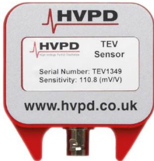
The HVPD TEV sensor is a small-size; electromagnetic sensor which can detect the high frequency radiation that is coupled onto earthed metal surfaces from 'local' partial discharge (PD) within switchgear, bushings and other plant.
