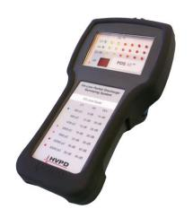
The PDS Air™ handheld partial discharge (PD) test unit is specially designed for the rapid PD 'screening' of large numbers of medium voltage (MV: 3.3–36 kV) assets. It is the only handheld PD test unit in the market to combine *three* PD sensors to detect PD activity in power cables, motors, generators, switchgear, and transformers.
